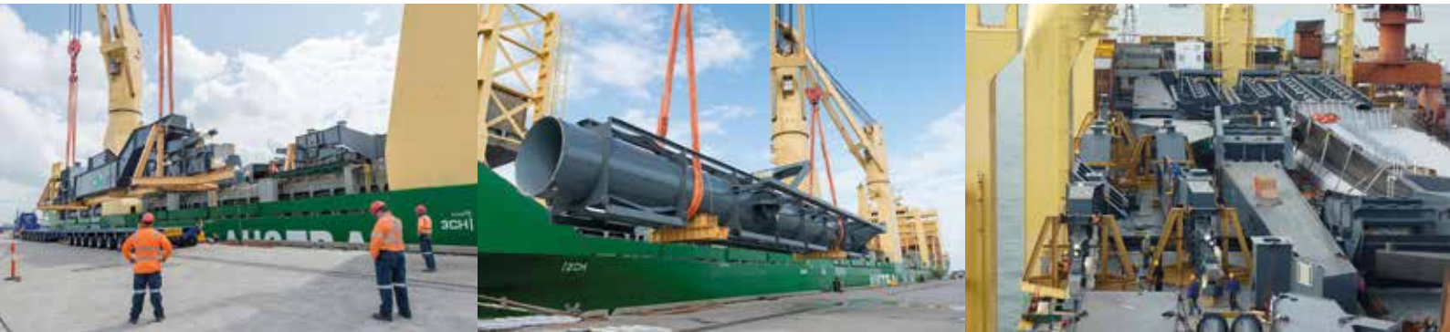
Discharge of scraper reclaimer modules in Australia NSW.
