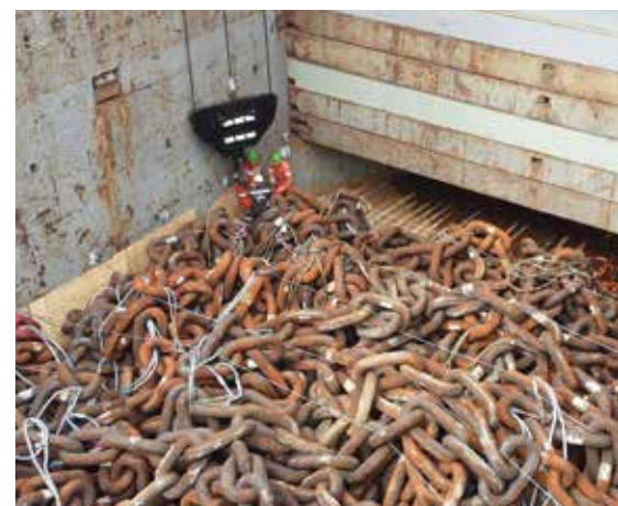
Lashing and securing of the mooring chains to prevent movement during the seavoyage.
