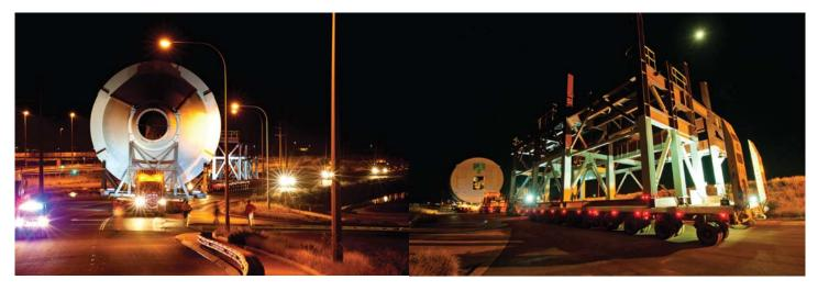
port. Eg. The Rom Bin with a weight of 310mT. Plus the Train Load Out bin measuring at 18m x 14m diameter and weighing 245mT plus the support structure measuring 21m x 14m diameter and weighing 175mT. This project required a significant amount of communication and co-ordination between NMT, vessel operators, Port Hedland Port Authority, main roads of Western Australia and Horizon Energy to deliver all cargo from vessel to site in a safe and timely manner.
